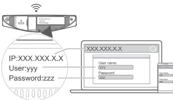
You can configure the router using the web-based management page. Please refer to the label on the bottom of the router for the default IP address, user name, and password.
